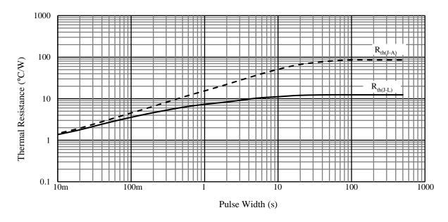
Figure 8. Typical Transient Thermal Resistance Characteristics
