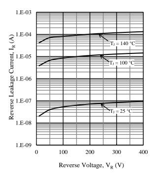
Figure 7. Typical Characteristics: I<sub>R</sub> vs. V<sub>R</sub>
