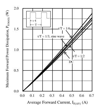
Figure 4.  $P_{F(MAX)}$  vs.  $I_{F(AV)}$  ( $T_J = 140$  °C)
