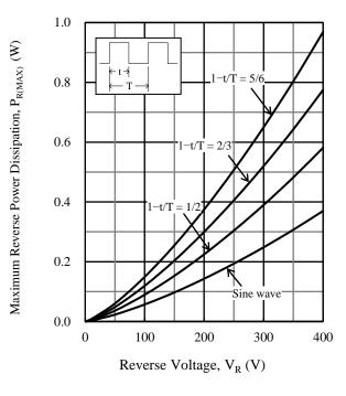
Figure 5.  $P_{R(MAX)}$  vs.  $V_R$  ( $T_J = 140$  °C)
