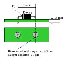
Figure 1. Lead Temperature Measurement Conditions
