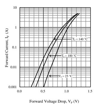
Figure 6. Typical Characteristics: I<sub>F</sub> vs. V<sub>F</sub>
