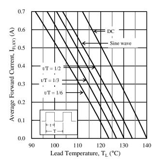
Figure 3.  $I_{F(AV)}$  vs.  $T_L^{(2)}$  ( $T_J = 140$  °C,  $V_R = 400$  V)
