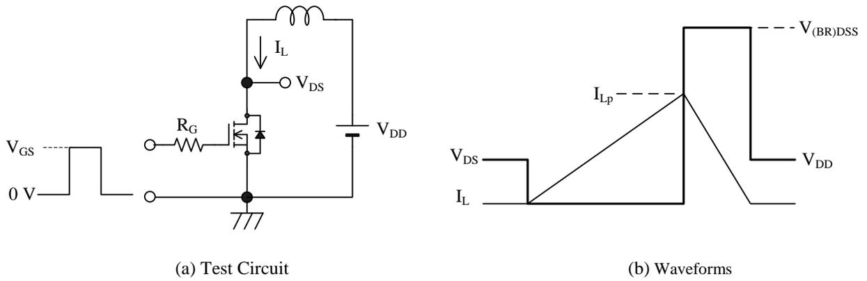
Figure 1 Unclamped Inductive
