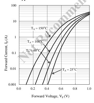
Figure 3-14  $V_F$  –  $I_F$  Typical Characteristics
