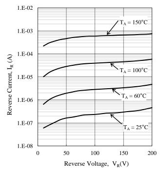
Figure 3-15  $V_R - I_R$  Typical Characteristics
