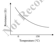
Figure 6-2 Reference characteristics of NTC thermistor
