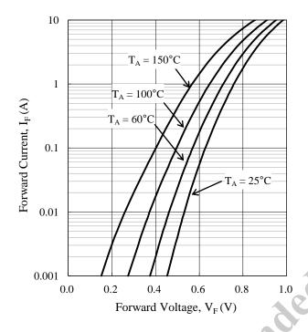
Figure 3-2 I<sub>F</sub> – V<sub>F</sub> Typical Characteristics
