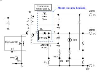
Figure 6-7 Reference circuit with FMKS series in the multi-output flyback converter circuit
