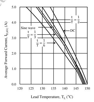
Figure 3-7  $I_{F(AV)} - T_L (V_R = 200 \text{ V})$
