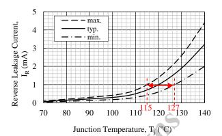
Figure 6-6 Temperature detection range at  $I_R$ = 1.0mA
