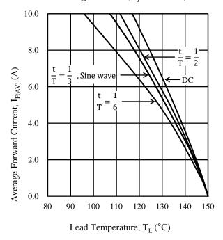
Figure 3-12  $I_{F(AV)} - T_L (V_R = 0 V)$
