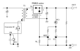
Figure 6-5 Reference temperature detection circuit with FMKS series.
