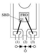
Figure 6-3 Internal structure of FMKS series
