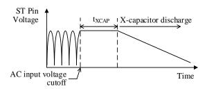
Figure 8-13. Operational Waveform at X-capacitor Discharge
