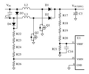
Figure 8-4. VREF and VSEN Pins and Their Peripheral Circuit
