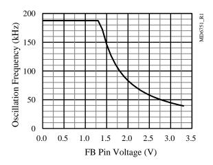
Figure 8-19. VGH/VGL Pin Oscillation Frequency vs. FB Pin Voltage
