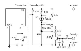
Figure 8-20. Standby Signal Input Circuit
