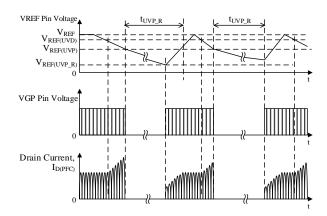
Figure 8-17. PFC UVP Operational Waveforms
