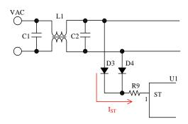
Figure 8-12. ST Pin and Its Peripheral Circuit
