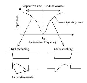
Figure 8-26. Operating Area of Resonant Power Supply
