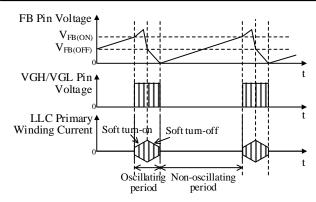
Figure 8-22. Operational Waveforms in Burst Oscillation Mode
