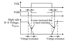
Figure 8-23. Waveforms When ZVS Failure Occurs
