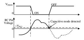
Figure 8-28. High-side Capacitive Mode Detection
