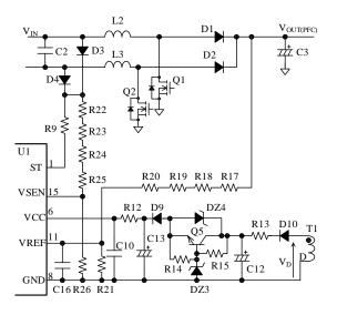
Figure 8-8. VCC Pin and Its Peripheral Circuit
