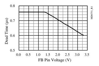
Figure 8-25. Dead Time vs. FB Pin Voltage
