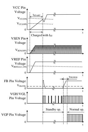
Figure 8-9. Operational Waveforms at Startup
