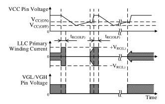
Figure 8-29. Operational Waveforms of LCC\_OCP and LCC\_OLP
