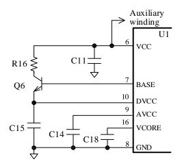
Figure 8-3. Power Stage and Its Peripheral Circuit
