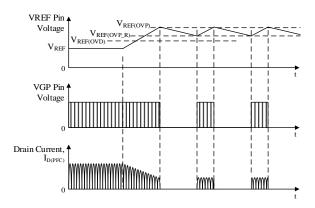
Figure 8-16. PFC\_OVP Operational Waveforms
