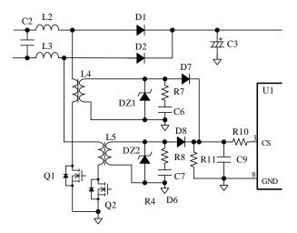
Figure 8-1. CS Pin and Its Peripheral Circuit
