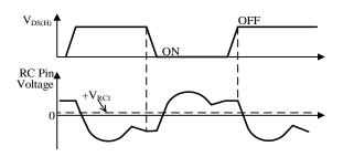
Figure 8-27. RC Pin Voltage Waveform in Inductive Area
