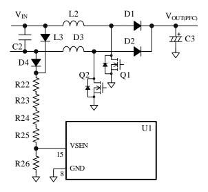
Figure 8-14. VSEN Pin and Its Peripheral Circuit
