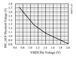
Figure 8-15. PFC\_OCP Threshold Voltage vs. VSEN Pin Voltage (Peak)
