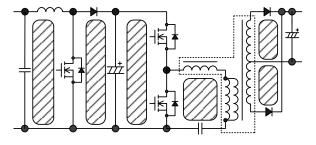
Figure 10-1. High-frequency Current Loop
