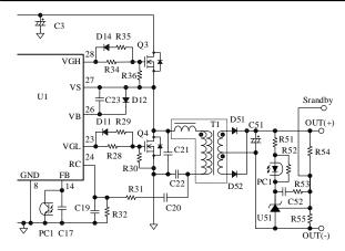
Figure 8-18. FB Pin and Its Peripheral Circuit
