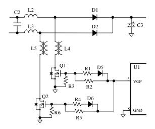
Figure 8-2. VGP Pin and Its Peripheral Circuit
