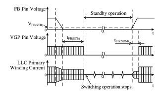
Figure 8-21. Operational Waveforms in Standby Mode
