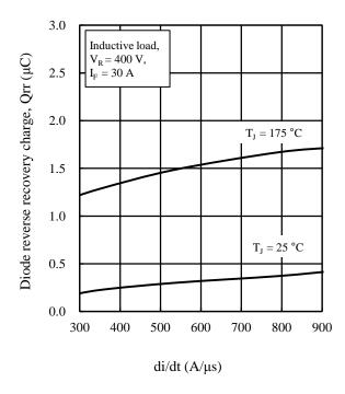
Figure 26. Diode Reverse Recovery Charge vs. di/dt
