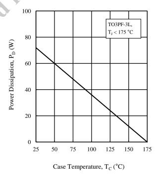
Figure 5. Power Dissipation vs. Case Temperature
