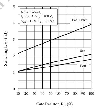
Figure 21. Switching Loss vs. Gate Resistor
