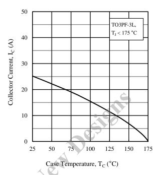
Figure 7. Collector Current vs. Case Temperature
