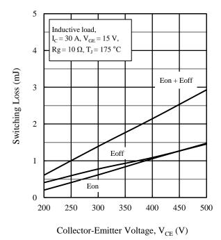
Figure 22. Switching Loss vs. Collector-Emitter Voltage
