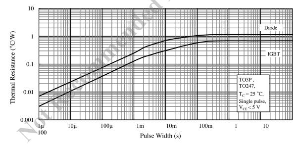
Figure 28. Transient Thermal Resistance
