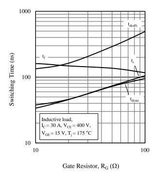
Figure 18. Switching Time vs. Gate Resistor
