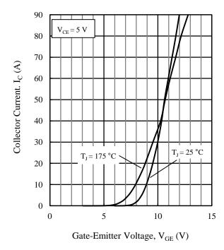
Figure 10. Transfer Characteristics
