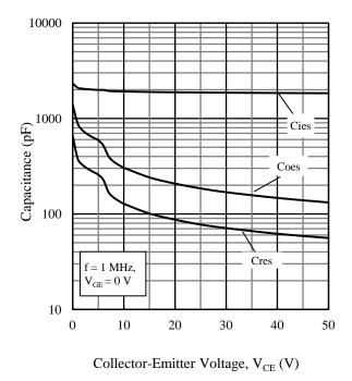
Figure 14. Capacitance Characteristics
