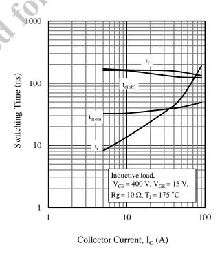
Figure 17. Switching Time vs. Collector Current
