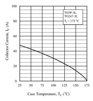
Figure 6. Collector Current vs. Case Temperature
