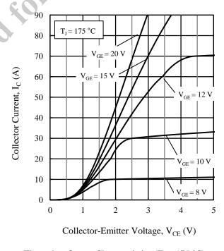
Figure 9. Output Characteristics ( $T_J = 175$  °C)
