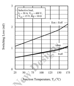
Figure 19. Switching Loss vs. Junction Temperature
