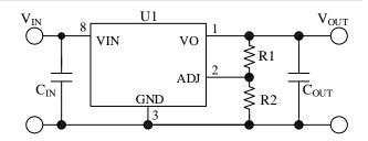
Figure 13-1. ADJ Pin Peripheral Circuit
