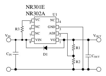
Figure 10-1. Typical Application (Output On/Off Function Disabled)
