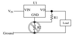
Figure 14-2. Output Voltage Setting (Do not connect R2.)
