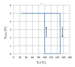
Figure 6-7. VC Pin Output On/Off Characteristics
