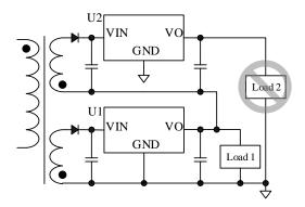
Figure 14-1. Stacked on Loads (Do not connect Load 2.)
