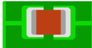
fig. 28 Improper Pattern Example
