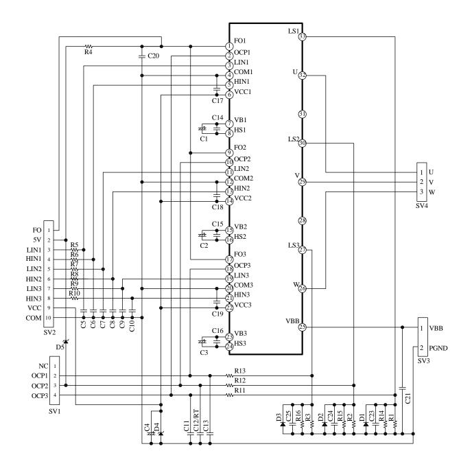
Figure 16-3. Circuit Diagram of PCB Pattern Layout Example
