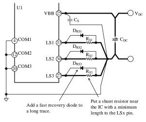
Figure 12-7. Connections to LSx Pin
