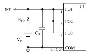
Figure 12-12. All-phase Shutdown Circuit
