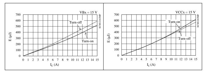
Figure 15-46. High-side Switching Loss ( $T_J = 125 \ ^{\circ}C$ )
