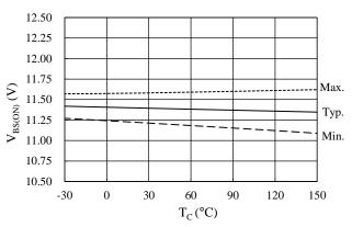
Figure 15-6. Logic Operation Start Voltage, V<sub>BS(ON)</sub> vs.  $T_{C}$
