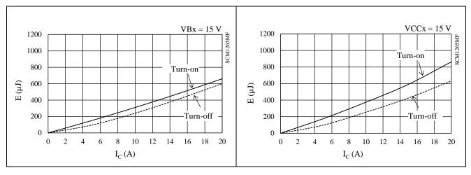
Figure 15-48 High-side Switching Loss ( $T_J = 25 \text{ °C}$ )
