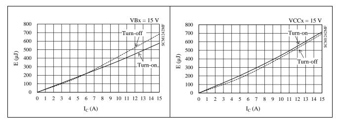
Figure 15-42. High-side Switching Loss ( $T_J = 125 \text{ °C}$ )
