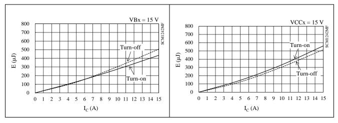
Figure 15-40 High-side Switching Loss ( $T_J = 25 \text{ °C}$ )
