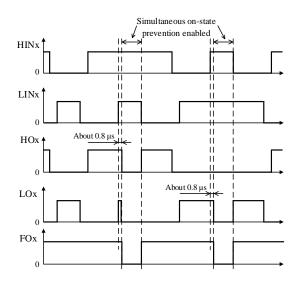
Figure 12-17. Operational Waveforms of Simultaneous On-state Prevention
