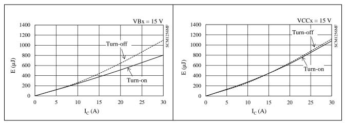
Figure 15-52. High-side Switching Loss ( $T_J = 25 \ ^{\circ}C$ )
