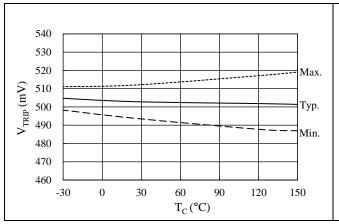
Figure 15-23. OCP Threshold Voltage, V<sub>TRIP</sub> vs. T<sub>C</sub>
