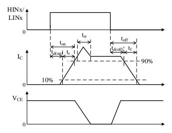
Figure 3-2. Switching Characteristics Definitions
