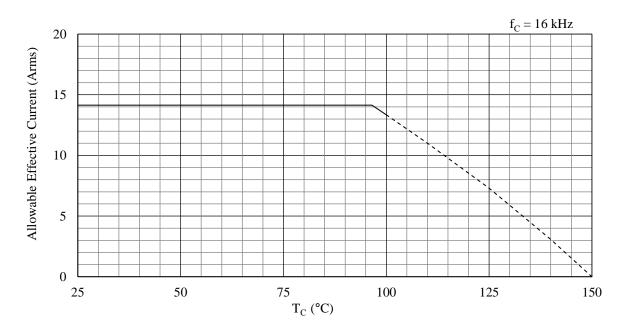
Figure 15-61. Allowable Effective Current ( $f_C = 16$  kHz): 20 A Devices
