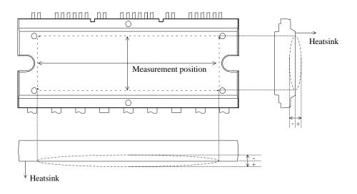
Figure 4-1. Flatness Measurement Position
