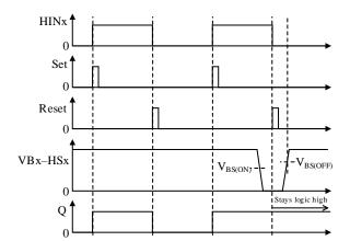
Figure 12-3. Waveforms at VBx-HSx Voltage Drop
