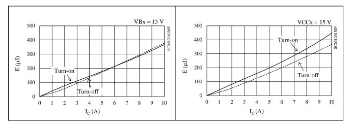
Figure 15-38. High-side Switching Loss ( $T_J = 125 \text{ °C}$ )
