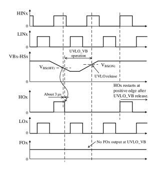
Figure 12-13. UVLO\_VB Operational Waveforms
