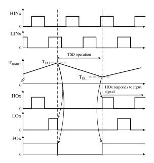
Figure 12-18. TSD Operational Waveforms
