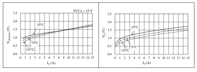
Figure 15-30. IGBT V<sub>CE(SAT)</sub> vs. I<sub>C</sub>
