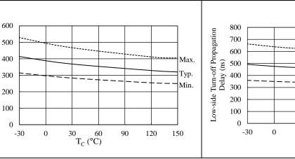
Figure 15-18. Low-side Turn-off Propagation Delay vs.  $T_C$  (from LINx to LOx)
