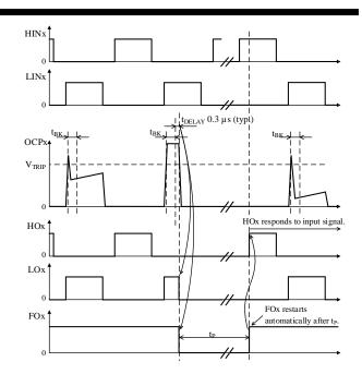
Figure 12-16. OCP Operational Waveforms
