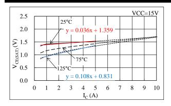
Figure 14-1. Linear Approximate Equation of  $V_{CE(SAT)}$  vs. I<sub>C</sub> Curve
