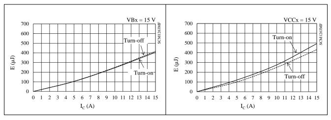
Figure 15-44 High-side Switching Loss ( $T_J = 25 \text{ °C}$ )
