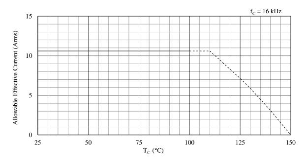
Figure 15-59. Allowable Effective Current ( $f_C = 16 \text{ kHz}$ ): 15 A Devices
