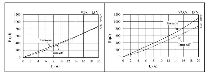
Figure 15-50. High-side Switching Loss ( $T_J = 125 \text{ °C}$ )
