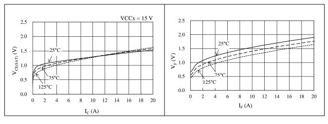
Figure 15-32. IGBT V<sub>CE(SAT)</sub> vs. I<sub>C</sub>
