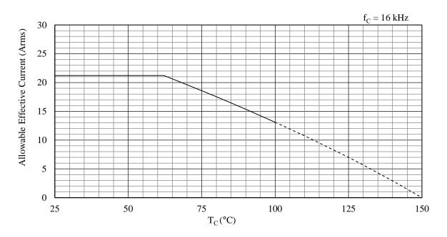
Figure 15-63. Allowable Effective Current ( $f_C = 16 \text{ kHz}$ ): 30 A Devices
