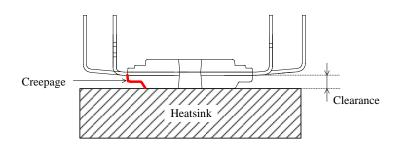
Figure 5-1. Insulation Distance Definitions
