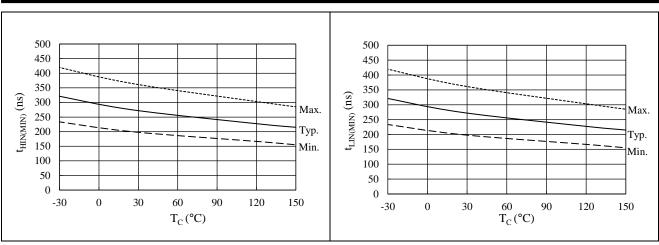
Figure 15-19. Minimum Transmittable Pulse Width for High-side Switching,  $t_{HIN(MIN)}$  vs.  $T_C$
