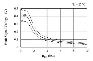
Figure 12-10. Fault Signal Voltage vs. Pull-up Resistor, R<sub>FO</sub>
