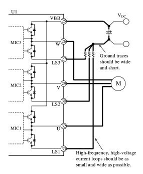
Figure 13-1. High-frequency, High-voltage Current Paths
