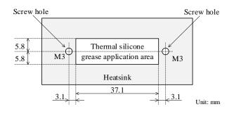
Figure 13-2. Reference Application Area for Thermal Silicone Grease
