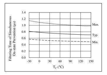
Figure 15-27. Filtering Time of Simultaneous On-state Prevention vs. T<sub>C</sub>
