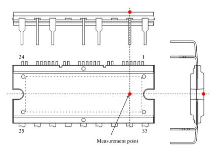
Figure 3-1. Case Temperature Measurement Point
