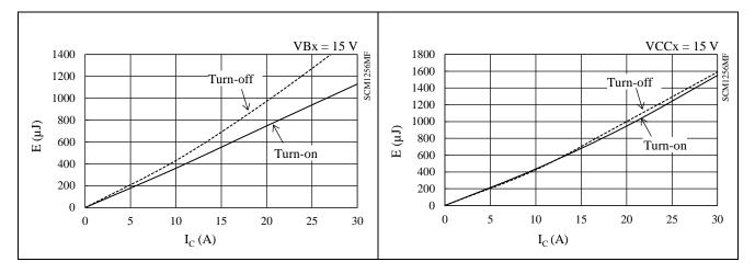
Figure 15-54. High-side Switching Loss ( $T_J = 125 \text{ °C}$ )
