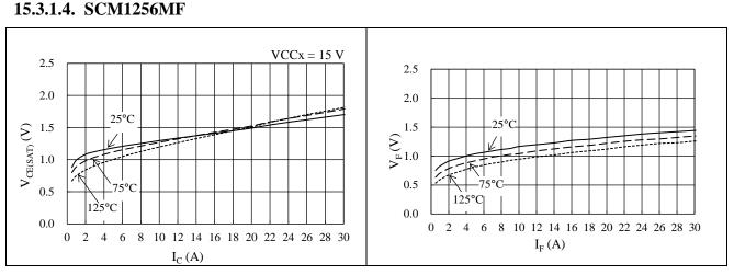
Figure 15-34. IGBT V<sub>CE(SAT)</sub> vs. I<sub>C</sub>
