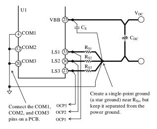
Figure 12-4. Connections to Logic Ground
