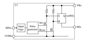
Figure 12-2. Internal Level-shifting Circuit
