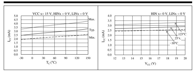
Figure 15-1. Logic Supply Current in 3-phase Operation, Figure 15-2. Logic Supply Current in 3-phase Operation, I<sub>CC</sub> vs. T<sub>C</sub>
