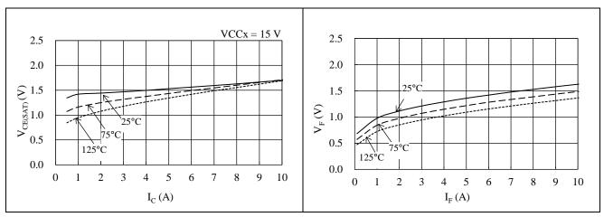
Figure 15-28. IGBT V<sub>CE(SAT)</sub> vs. I<sub>C</sub>
