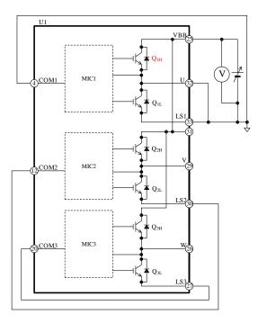
Figure 13-3. Typical Measurement Circuit for High-side Transistor (Q<sub>1H</sub>) in U-phase
