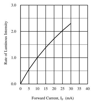
Figure 3. Rate of Luminous Intensity vs. I<sub>F</sub>
