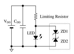
Example of Adding Zener Diodes (ZD1, ZD2:  $V_Z = 7 V \text{ to } 8 V$ )
