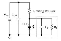
Example of Adding Filter ( $C_P \ge 0.01 \mu F$ ,  $R_P = 10 k\Omega$ )
