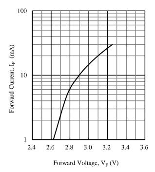
Figure 2. I<sub>F</sub> vs. V<sub>F</sub>
