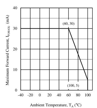
Figure 1. I<sub>F(MAX)</sub> vs. T<sub>A</sub>
