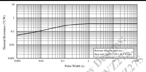
Figure 7. Typical Transient Thermal Resistance<sup>(3)</sup>
