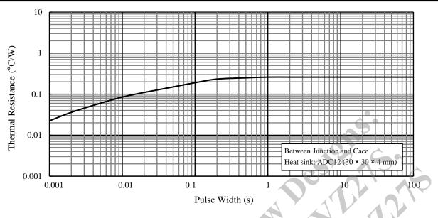
Figure 17. Typical Transient Thermal Resistance<sup>(7)</sup>
