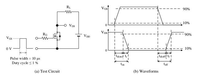
Figure 18. Resistive Load Switching Time Test
