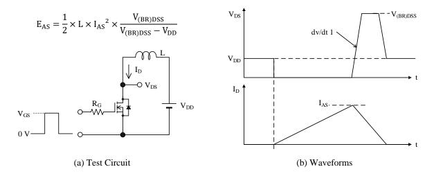
Figure 16. Avalanche Energy and dv/dt1 Test
