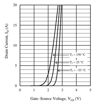
Figure 6. Typical Characteristics:  $I_D \text{ vs. } V_{GS} \text{ (V}_{DS} = 10 \text{ V)}$
