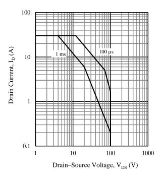
Figure 4. Typical Characteristics: Safe Operating Area (Single Pulse,  $T_{J}\!=\!25~^{\circ}\text{C})$
