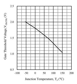
Figure 7. Typical Characteristic:  $V_{GS(TH)}$  vs.  $T_J$  ( $V_{DS} = 10$  V,  $I_D = 1$  mA)
