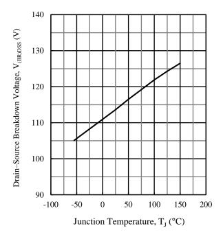
Figure 12. Typical Characteristic:  $V_{(BR)DSS}$  vs.  $T_J$  ( $I_D = 10$  mA,  $V_{GS} = 0$  V)
