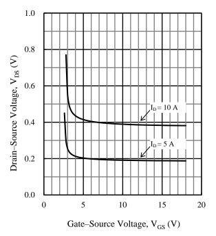
Figure 14. Typical Characteristics:  $V_{DS}$  vs.  $V_{GS}$  ( $V_{DS}$  = 10 V)
