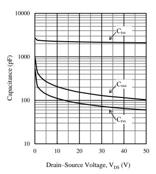
Figure 11. Typical Characteristics: Capacitance vs.  $V_{DS}$  (f = 1 MHz,  $V_{GS}$  = 0 V)
