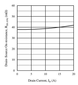
Figure 8. Typical Characteristic:  $R_{DS(ON)}$  vs.  $I_D$  (V  $_{GS}=10$  V,  $T_J=25$   $^{\circ}C)$
