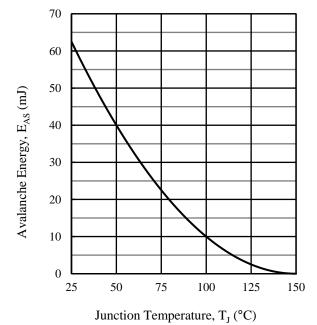
Figure 3. E<sub>AS</sub> vs. T<sub>J</sub> (Single Pulse)
