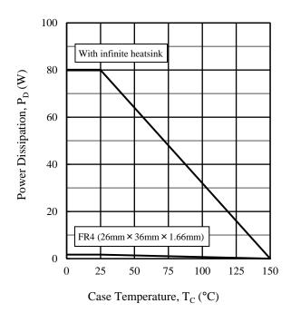
$\begin{array}{cc} Figure \ 1. & P_D \ vs. \ T_C \\ (All \ Power \ MOSFETs \ Operating) \end{array}$
