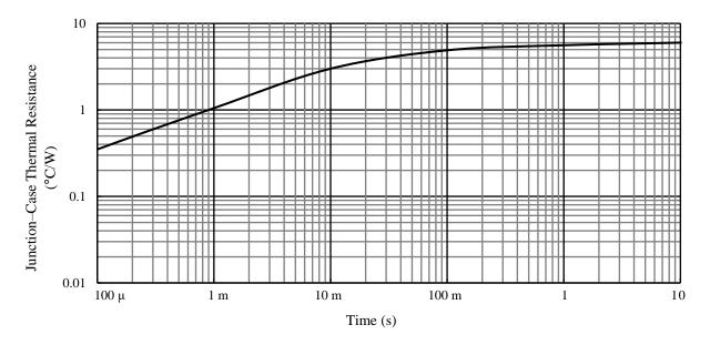
Figure 15. Transient Thermal Resistance Characteristic (Single Pulse,  $T_C = 25$  °C,  $V_{DS} < 10$  V)
