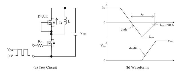
Figure 17. Diode Reverse Recovery Time Test
