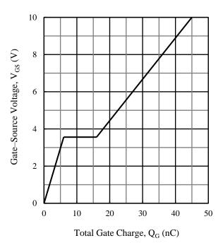
Figure 13. Typical Characteristic:  $V_{GS}$  vs.  $Q_G$  ( $I_D$  = 5 A,  $V_{DD}$   $\approx$  50 V)
