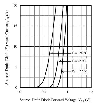
Figure 10. Typical Characteristics:  $I_S$  vs.  $V_{SD}$  ( $V_{GS} = 0$  V)
