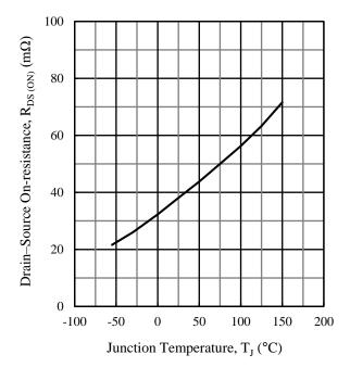
Figure 9. Typical Characteristic:  $R_{DS(ON)}$  vs.  $T_J$  ( $V_{GS} = 10$  V,  $I_D = 5$  A)
