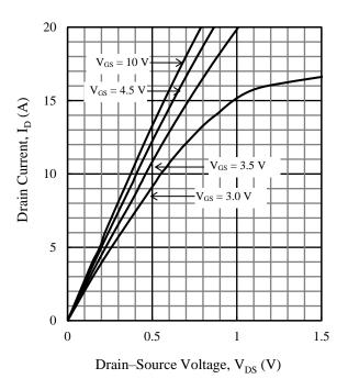
Figure 5. Typical Characteristics:  $I_D$  vs.  $V_{DS}$   $(T_J = 25 \, ^{\circ}C)$
