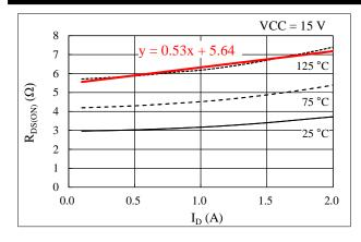
Figure 14-2. Linear Approximate Equation of  $R_{DS(ON)}$  vs.  $I_D$
