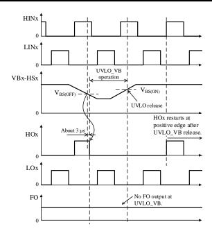
Figure 12-10. UVLO\_VB Operational Waveforms
