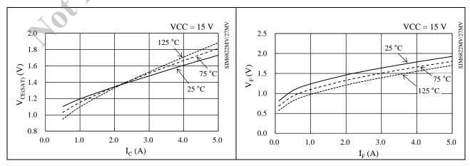
Figure 15-37. IGBT V<sub>CE(SAT)</sub> vs. I<sub>C</sub>
