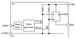
Figure 12-2. Internal Level-shifting Circuit
