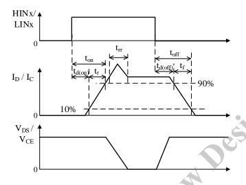
Figure 3-2. Switching Characteristics Definitions
