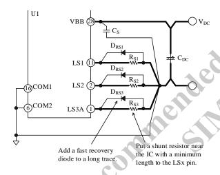
Figure 12-8. Connections to LSx Pin
