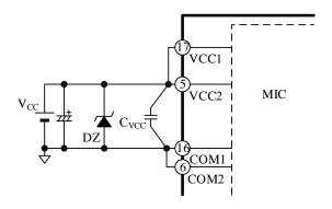
Figure 12-4. VCCx Pin Peripheral Circuit
