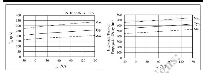
Figure 15-18. Input Current at High Level (HINx or LINx),  $I_{\rm IN}$  vs.  $T_{\rm C}$
