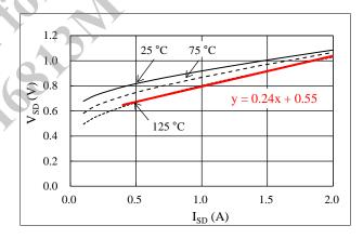
Figure 14-3. Linear Approximate Equation of  $V_{SD}$  vs.  $I_{SD}$
