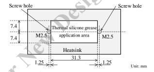
Figure 13-2. Reference Application Area for Thermal Silicone Grease
