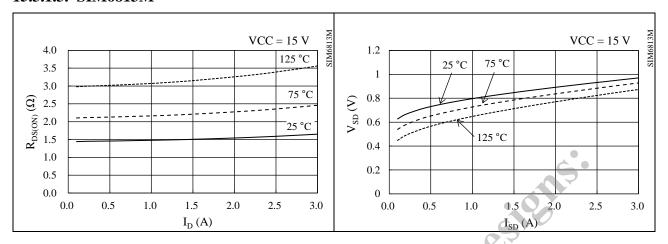
Figure 15-33. Power MOSFET R<sub>DS(ON)</sub> vs. I<sub>D</sub>
