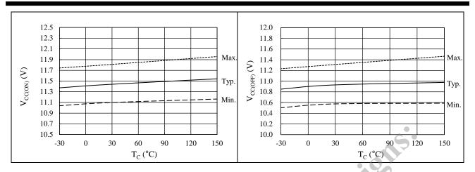
Figure 15-12. Logic Operation Start Voltage,  $V_{CC(ON)}$  vs.  $T_C$
