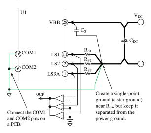
Figure 12-5. Connections to Logic Ground
