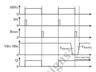
Figure 12-3. Waveforms at VBx–HSx Voltage Drop
