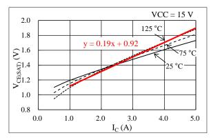
Figure 14-1. Linear Approximate Equation of  $V_{\text{CE(SAT)}}$  vs.  $I_{\text{C}}$
