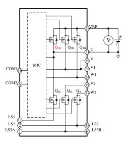
Figure 13-3. Typical Measurement Circuit for Highside Transistor ( $Q_{1H}$ ) in U-phase
