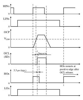
Figure 12-13. OCL Operational Waveforms (OCL = SD)
