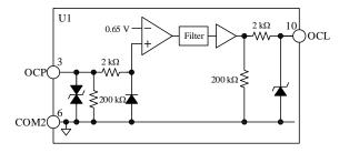
Figure 12-12. Internal Circuit of OCP and OCL Pins
