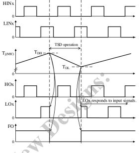
Figure 12-16. TSD Operational Waveforms
