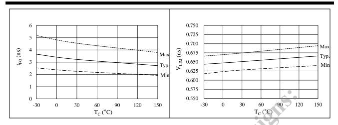
Figure 15-24. FO Pin Filtering Time vs. T<sub>C</sub>
