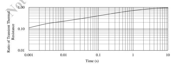
Figure 15-3. Transient Thermal Resistance: SIM6880M
