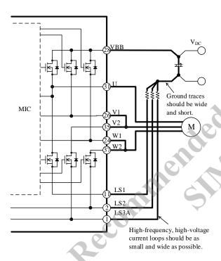
Figure 13-1. High-frequency, High-voltage Current Paths
