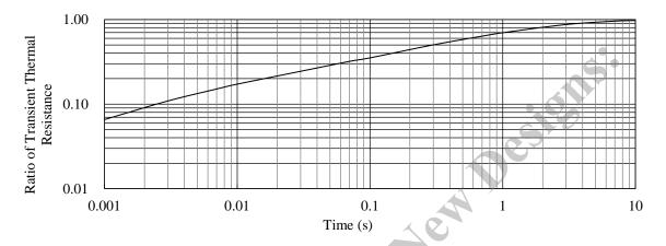
Figure 15-1. Transient Thermal Resistance: SIM6810M
