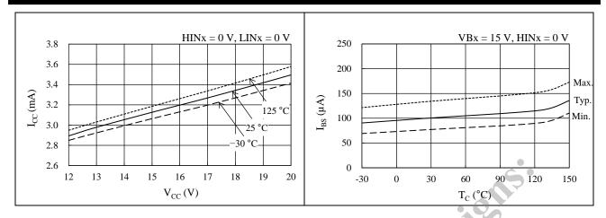
Figure 15-6. VCCx Pin Voltage,  $V_{CC}$  vs. Logic Supply Current,  $I_{CC}$
