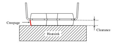
Figure 5-1. Insulation Distance Definitions
