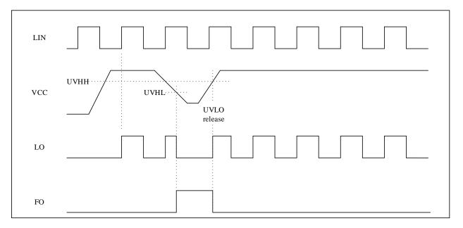
Figure 8-2. Low-side Undervoltage Lockout for Power Supply (UVLO\_VCC)
