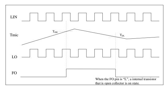
Figure 8-3. Thermal Detection (TD)
