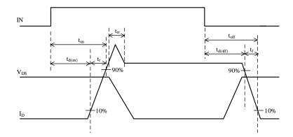
Figure 3-1. Switching Characteristics Definitions
