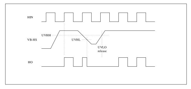
Figure 8-1. High-side Undervoltage Lockout for Power Supply (UVLO\_VB)
