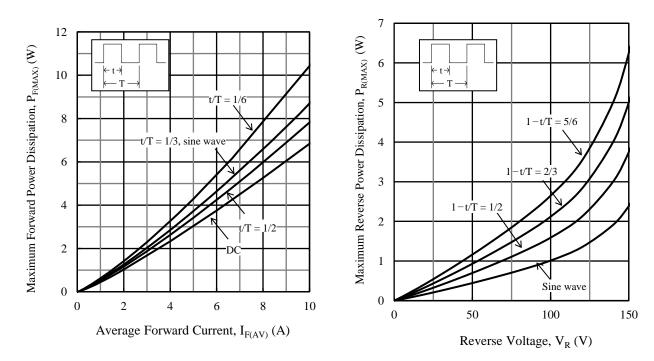
Figure 5.  $P_{F(MAX)}$  vs.  $I_{F(AV)}$  (T<sub>J</sub> = 150 °C)
