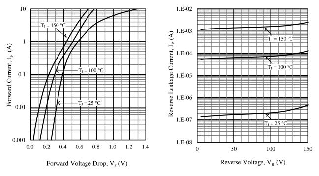
Figure 7. Typical Characteristics: I<sub>F</sub> vs. V<sub>F</sub>
