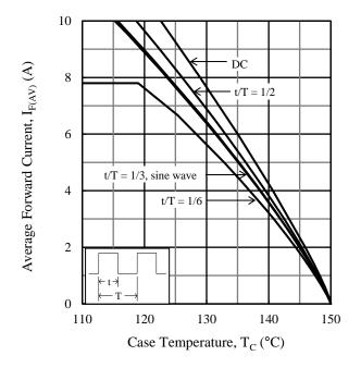
Figure 3.  $I_{F(AV)}$  vs.  $T_C$  ( $T_J = 150 \ ^\circ C$ ,  $V_R = 0 \ V$ )
