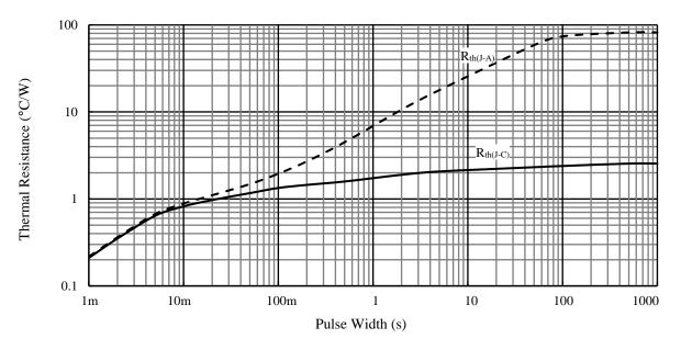
Figure 9. Typical Transient Thermal Resistance Characteristics
