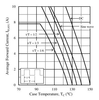
Figure 4.  $I_{F(AV)}$  vs.  $T_C$  ( $T_J = 150$  °C,  $V_R = 150$  V)
