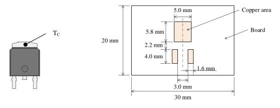
Figure 1. Case Temperature Measurement Point
