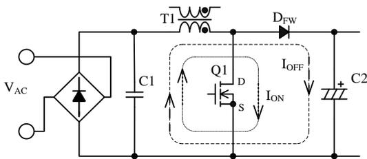
Figure 8-1. PFC Circuit
