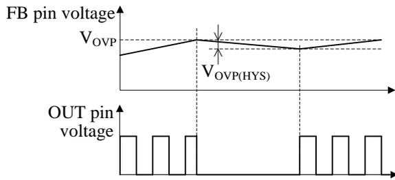
Figure 8-13. OVP Waveforms
