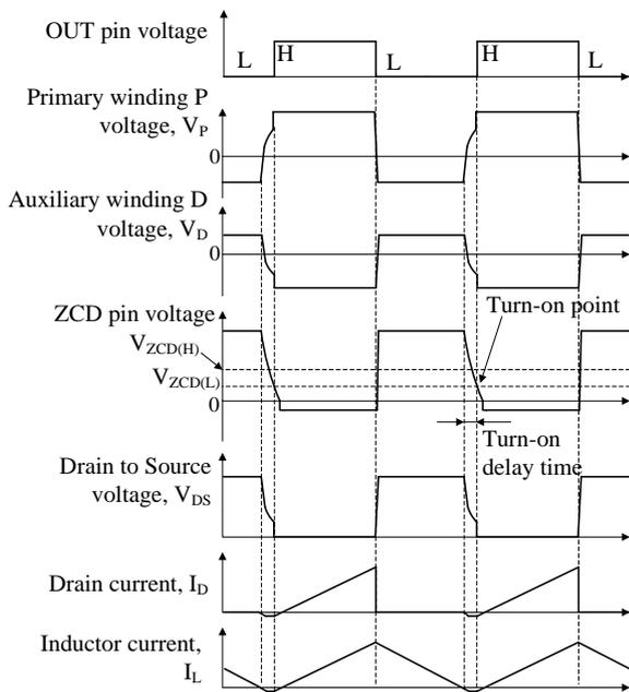
Figure 8-10. Zero Current Detection Waveform
