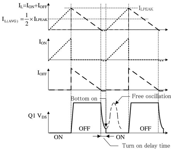
Figure 8-2. CRM Operation and Bottom On Operation
