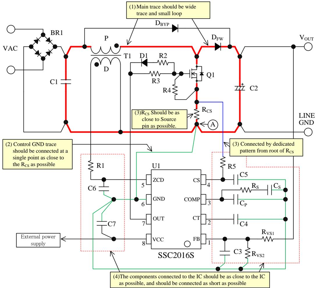
Figure 9-6. Example of Connection of Peripheral Component
