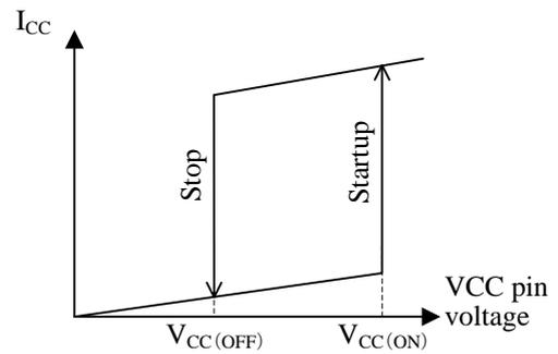
Figure 8-6. Relationship between VCC Pin Voltage and  $I_{CC}$
