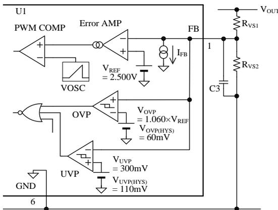
Figure 8-14. The FB Pin Peripheral Circuit and Internal Circuit.
