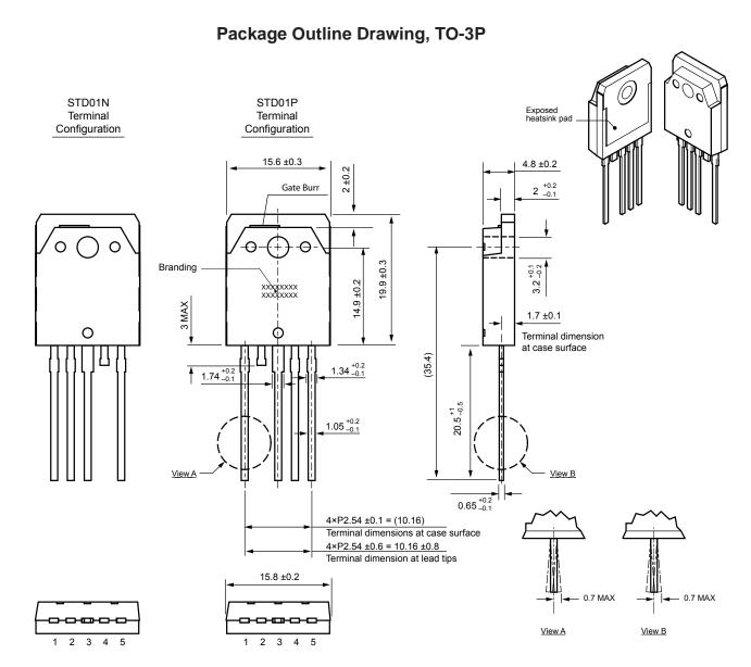
Gate burr: 0.3 mm (max.), mold flash may appear at opposite side Terminal core material: Cu
