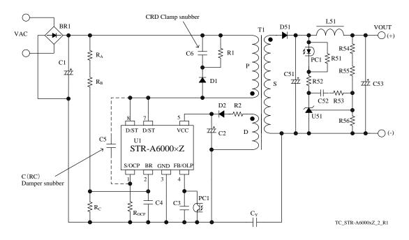
Figure 6-1 Typical application (enabled Brown-In/Brown-Out Function, DC line detection)
