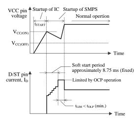
Figure 9-6 V<sub>CC</sub> and I<sub>D</sub> behavior during startup
