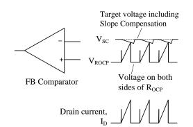
Figure 9-8 Drain current, I<sub>D</sub>, and FB comparator operation in steady operation
