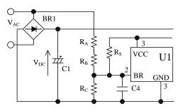
Figure 9-13 AC line detection
