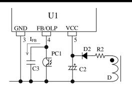
Figure 9-17 FB/OLP pin peripheral circuit
