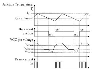
Figure 9-20 TSD operational waveforms
