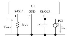
Figure 9-7 FB/OLP pin peripheral circuit
