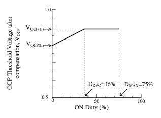
Figure 9-16 Relationship between ON Duty and Drain Current Limit after compensation
