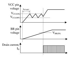
Figure 9-3 Startup operation (With Brown-In / Brown-Out Function)
