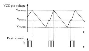
Figure 9-19 OVP operational waveforms
