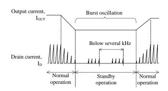
Figure 9-10 Auto Standby mode timing
