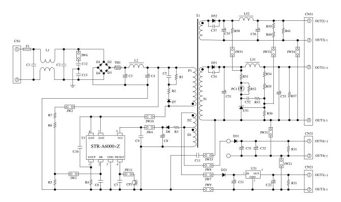
Figure 11-2 Circuit schematic for PCB circuit trace layout
