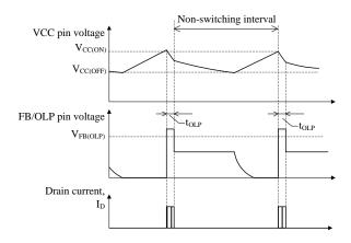
Figure 9-18 OLP operational waveforms
