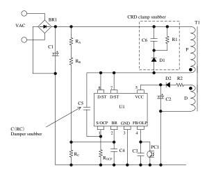
Figure 10-1 The IC peripheral circuit
