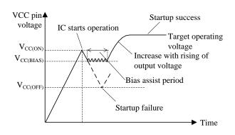
Figure 9-5 VCC pin voltage during startup period
