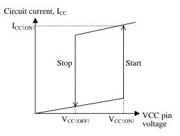
$\begin{array}{c} Figure \ 9-4 \quad Relationship \ between \\ VCC \ pin \ voltage \ and \ I_{CC} \end{array}$
