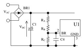
Figure 9-12 DC line detection
