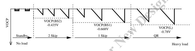
Fig.7-23 Transition diagram from no load to heavy load
