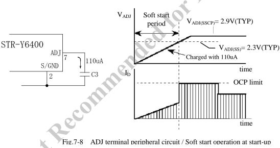
$V_{ADJ(SSCP)}$  is 2.9V (TYP) on the steady state condition.
