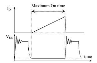
Fig.7-27 Maximum T<sub>ON</sub> period confirmation
