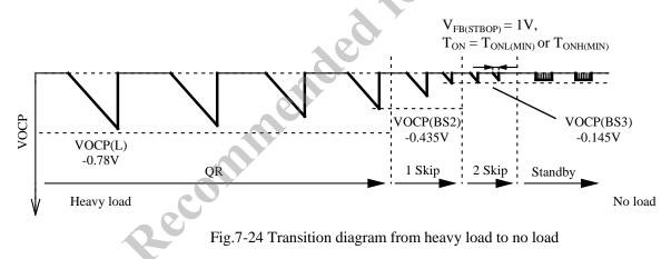
As the hysteresis is implemented for each mode switching of the increasing / decreasing load transitions, the oscillation is stable near the switching thresholds and the mode switching is achieved stably.
