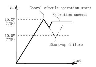
Fig.7-3  $V_{CC}$  behavior at startup
