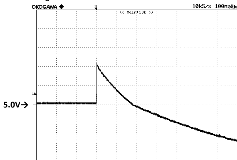
図16 過電圧波形 Fig.16 Over Voltage Waveform
