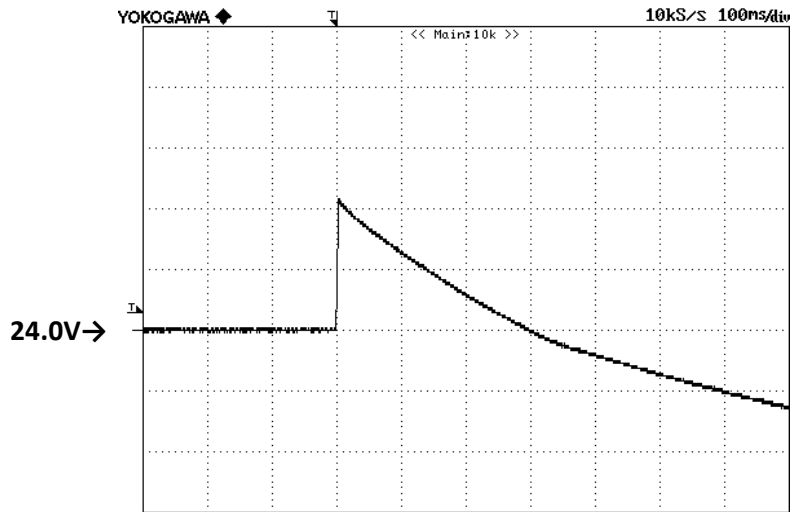
図16 過電圧波形 Fig.16 Over Voltage Waveform
