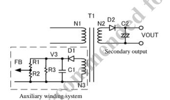
Regarding the operation of constant voltage control, if the secondary load decreases, voltage in the auxiliary winding system also increases as the output voltage increases, and voltage entered into the FB pin also increases. This voltage is negatively amplified by the error amplifier in the IC, so add a slope compensation signal to generate a target value of the FB Comparator.
