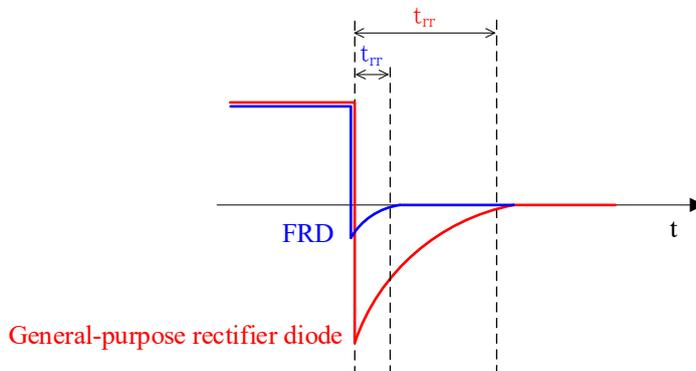
Figure 3-1. Comparison of Reverse Recovery Time,  $t_{rr}$
