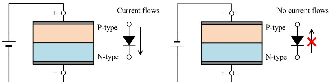
Figure 2-7. Direction to Apply Voltage
