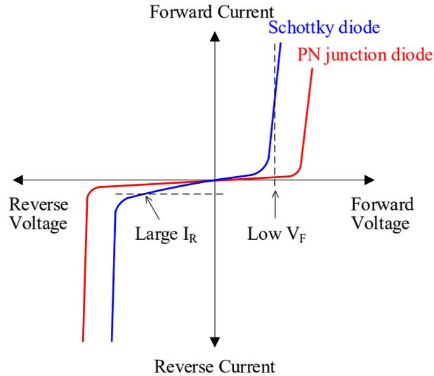
Figure 3-7. Static Characteristics Comparison
