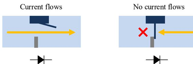
Figure 2-1. Schematic View of Diode
