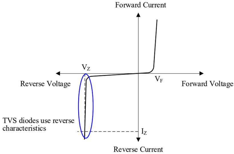
Figure 3-6. Diode Static Characteristics
