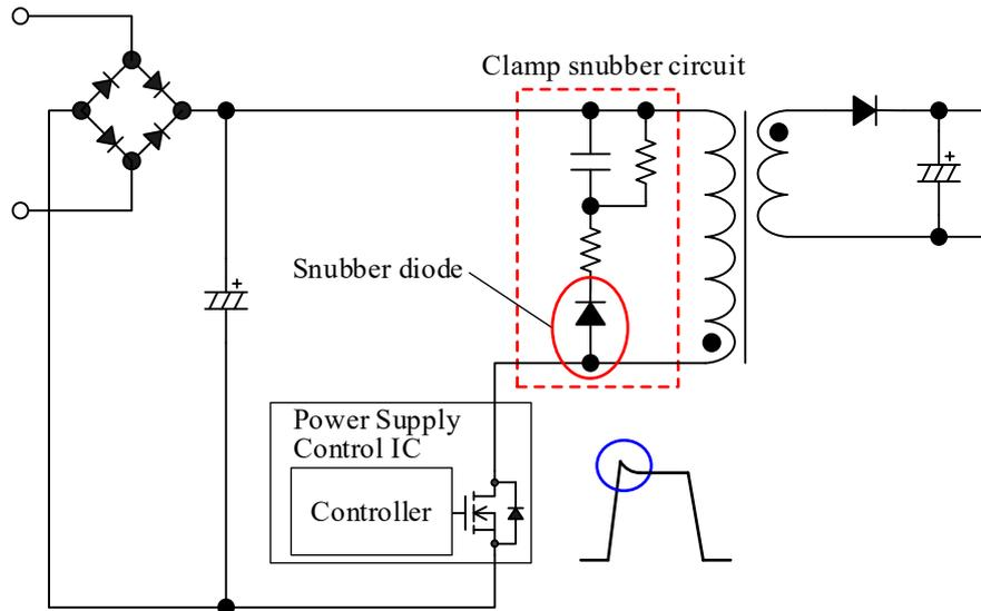
Figure 3-4. Clamp Snubber Circuit
