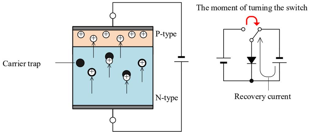
Figure 3-2. Carrier Trap
