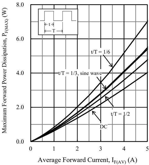
Figure 3.  $P_{F(MAX)}$  vs.  $I_{F(AV)}$  ( $T_J = 150\text{ }^\circ\text{C}$ )
