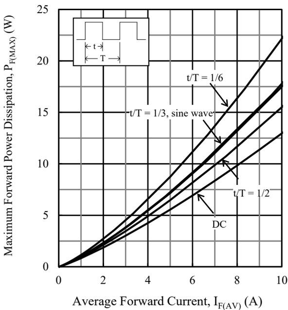
Figure 3.  $P_{F(MAX)}$  vs.  $I_{F(AV)}$  ( $T_J = 150\text{ }^\circ\text{C}$ )
