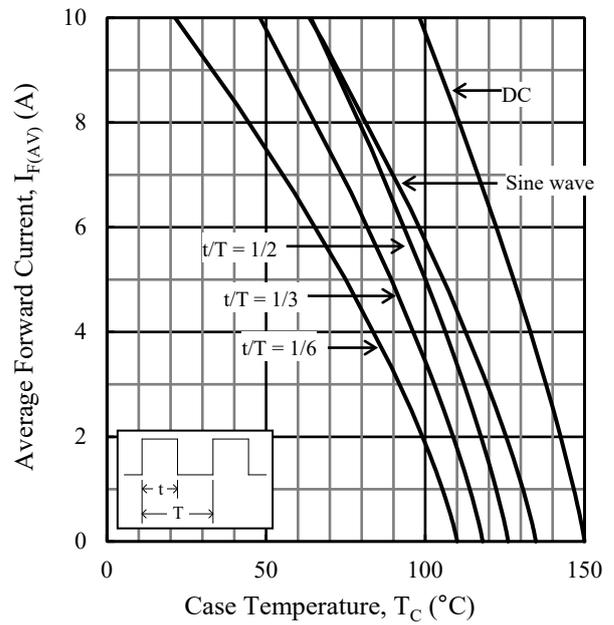
Figure 2.  $I_{F(AV)}$  vs.  $T_C$  ( $T_J = 150\text{ }^\circ\text{C}$ ,  $V_R = 400\text{ V}$ )
