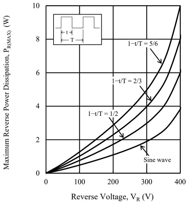
Figure 4.  $P_{R(MAX)}$  vs.  $V_R$  ( $T_J = 150\text{ }^\circ\text{C}$ )
