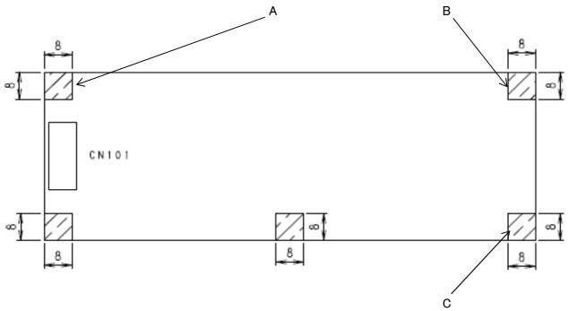
Use a small washer W sem screw M3 as the mounting screw.
