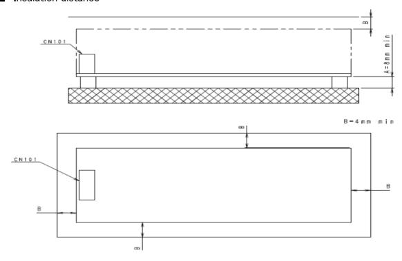
If a metal case is used, secure the dimensions of A and B for the separation between the power supply and the metal case.
