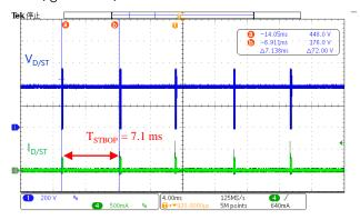
The burst oscillation period becomes long according to the power reduction.
