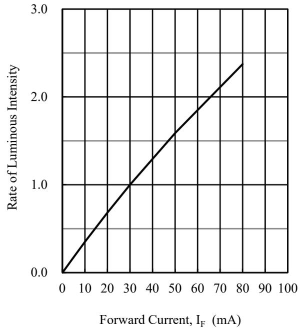
Figure 3. Rate of Luminous Intensity vs.  $I_F$
