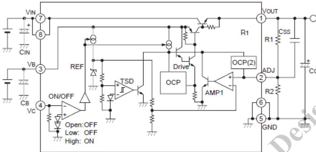
$C_{IN}$ ,  $C_B$ : Input Capacitor and Biased Capacitor (0.1 $\mu$ F - 10 $\mu$ F)
