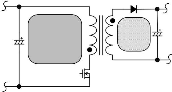
Figure 9-6. High Frequency Current Loops (Hatched Areas)
