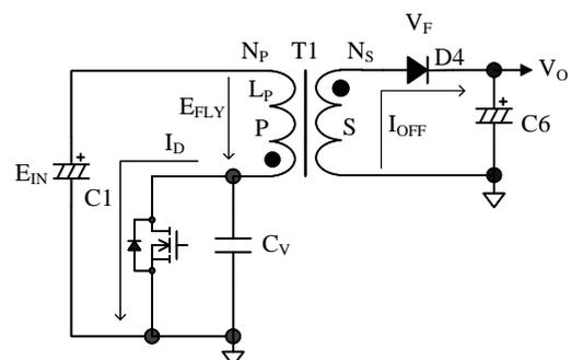
Figure 9-1. Quasi-resonant Circuit
